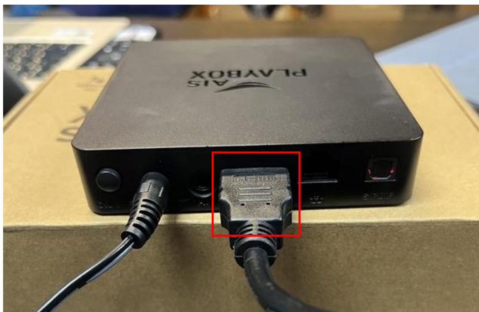
Image 2.2 How to connect HDMI cable to AIS PLAYBOX.
