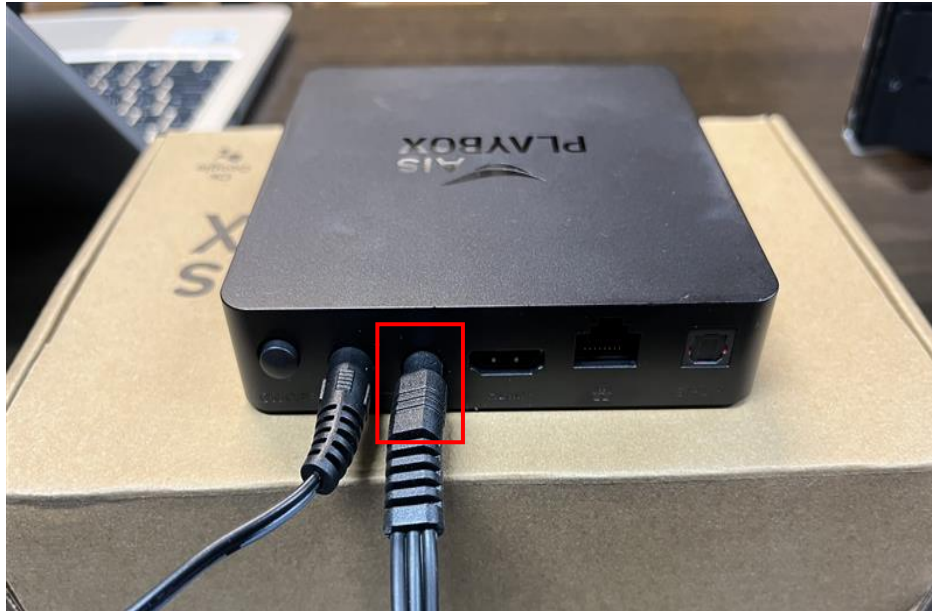
Image 2.1 How to connect the AV cable to the AIS PLAYBOX.
